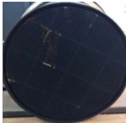
FIGURE 2. Appearance of a dirty filter element
